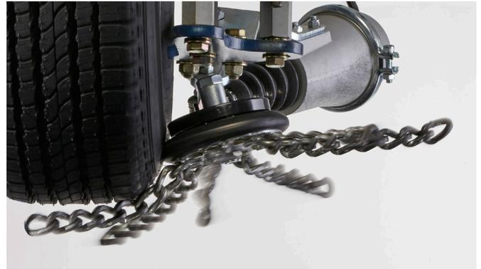
The twist allows the leading edges of the chain to dig or bite into the ice and snow
